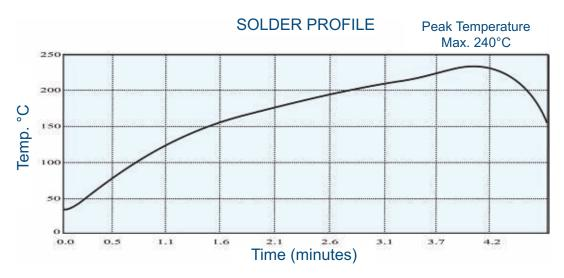
If acqueous cleaning is used for flux removal, bake parts at least 1 minute at 80°C maximum after water rinse.
