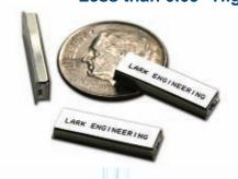
When size is critical, Lark is offering a full line of Ultra-Thin filters for the Commercial and Military markets. Lark's new Ultra-Thin package offers superior performance in less than 0.09" high package. The Ultra-Thin filter series offers low insertion loss and ultimate rejection levels of 60 dB while maintaining better than 1.5:1 VSWR. These units are lightweight and ruggedized for today's military applications.
